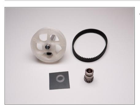
Get Wheel, Spacer, Bondtech drive gear and Belt
